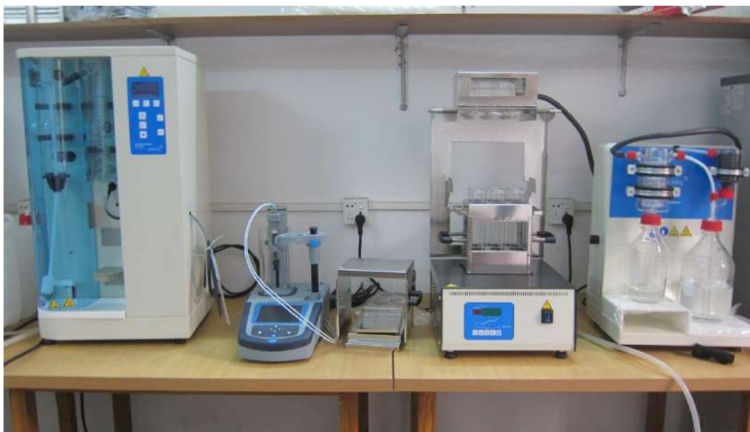
Kjeldahl Protein Analyzer of Food and Nutrition Lab, SST, BOU
